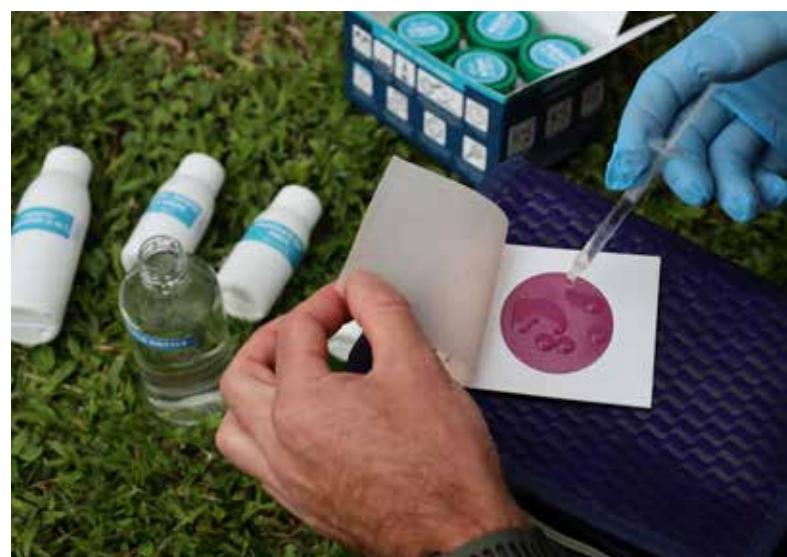
Figure 3: A water sample is being tested with AfriForum's field testing kit.
